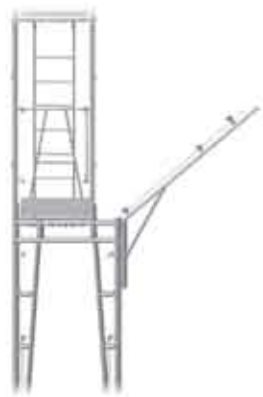
Facade scaffolding with protective front and pedestrian walkthrough
